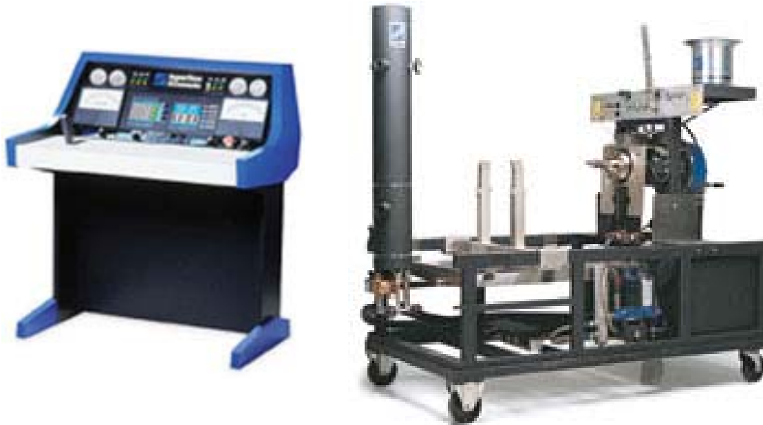
Figure 6 – Superflow Control Bench and Dynamometer
